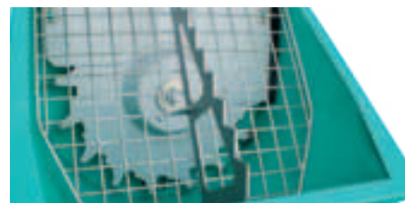
Hopper with grate and bag breaker (Standard version).
